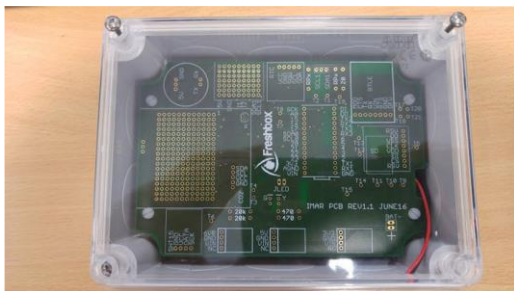
Fig. 5. Integrated sensors kit v 1.2 P.C.B. in housing
