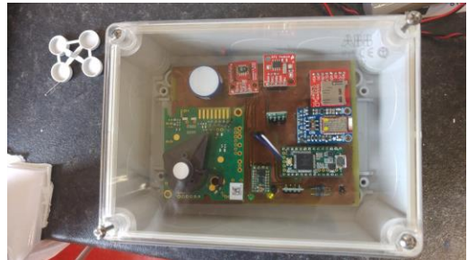
Fig. 4. Oxy4 etched P.C.B., populated with sensors and secured in housing.
